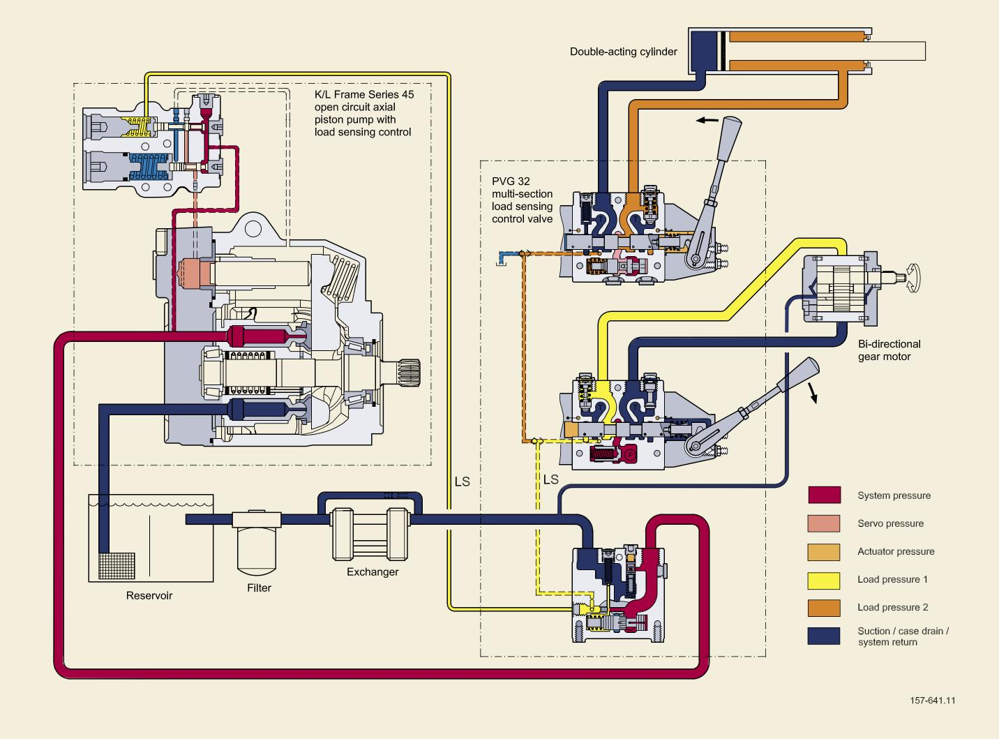
The modular design of the Sauer-Danfoss PVG 32 load sensing valve, accommodates future control variations and gives you an almost infinite number of configuration possibilities.
